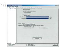
When connected, wireless connection status (data speed, signal strength, link quality ...etc.) will be displayed in wireless utility window. Click "Close" to hide the wireless adapter utility.
